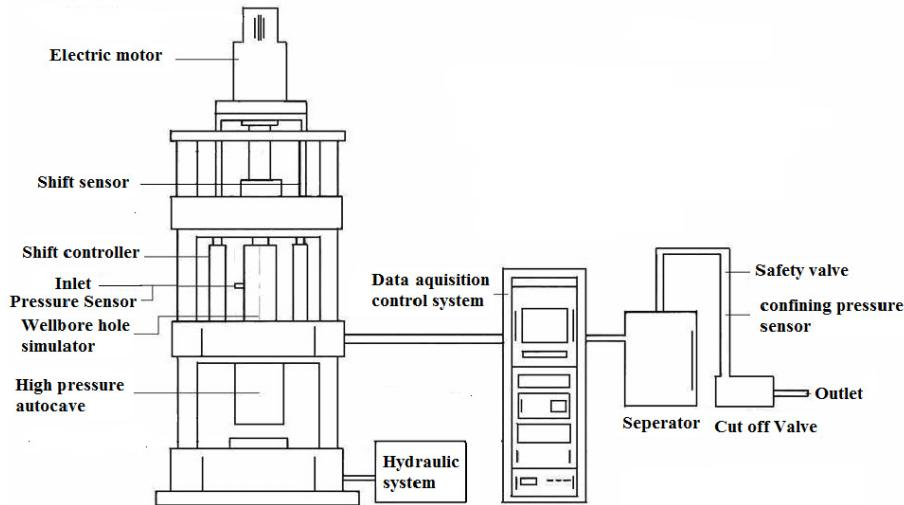
**FIG. 2:** The test device for jets breaking rock.
