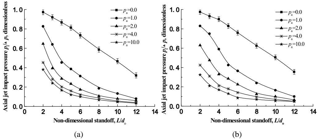
**FIG. 5:** The relation between axial jet impact pressure and nondimensional standoffs under different confining pressures. (a)  $\Delta p = 15.0$  MPa and (b)  $\Delta p = 20.0$  MPa.
