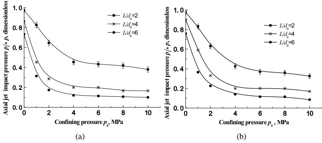
**FIG. 4:** The relationship between axial jet impact pressure and confining pressure at different nondimensional standoffs. (a)  $\Delta p = 15.0$  MPa and (b)  $\Delta p = 20.0$  MPa.
