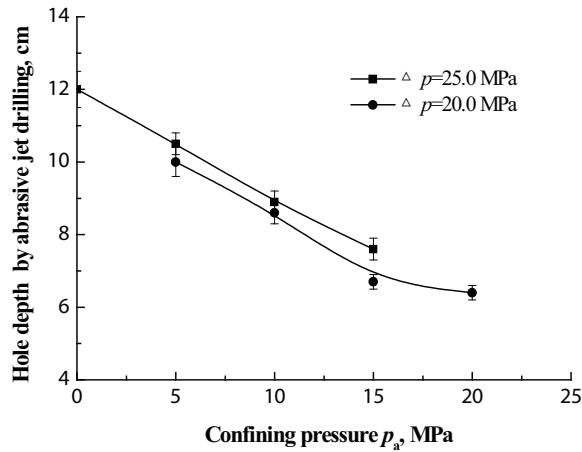
**FIG. 11:** Hole depth by abrasive jet drilling under different confining pressures.
