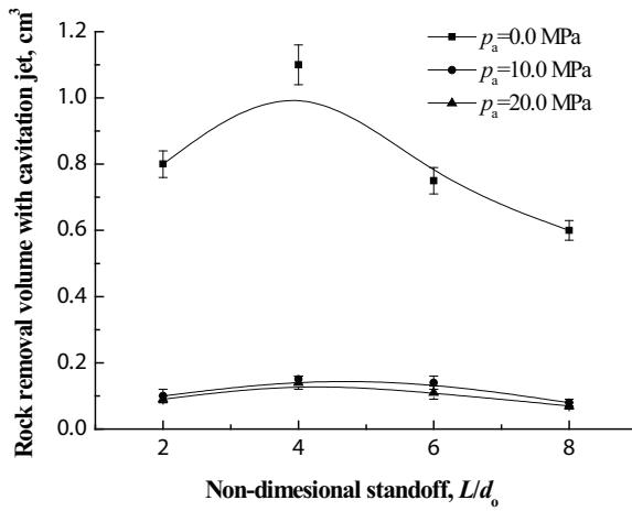
**FIG. 9:** Rock removal volume by the cavitating nozzle at different standoffs.
