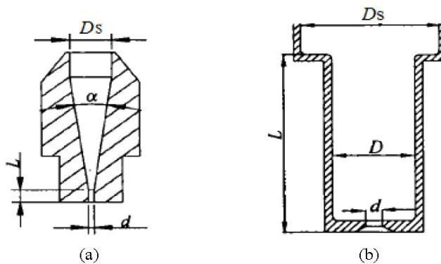
**FIG. 3:** Schematic diagram of nozzles for the test. (a) Conical nozzle and (b) cavitating nozzle.
