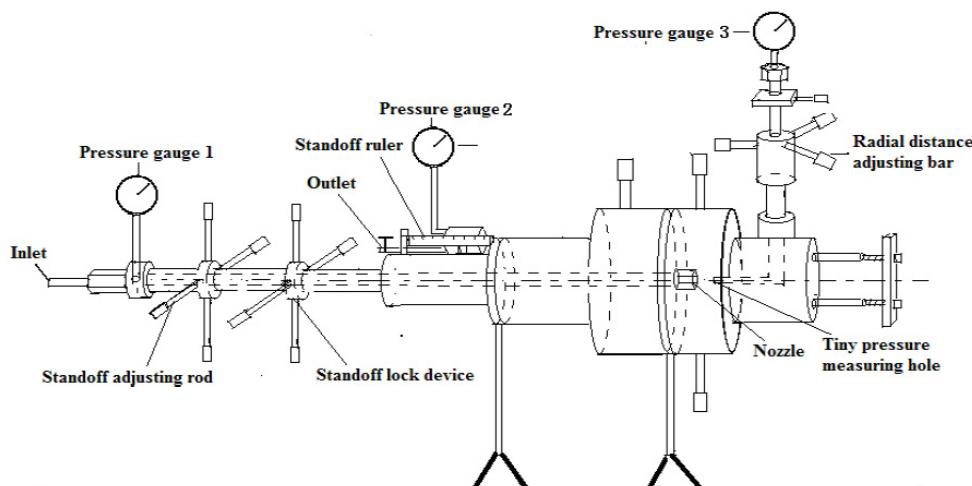
**FIG. 1:** The test device for measuring jet impact pressure.
