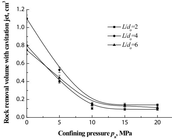
**FIG. 8:** Rock removal volume, the cavitating nozzle under different confining pressures.
