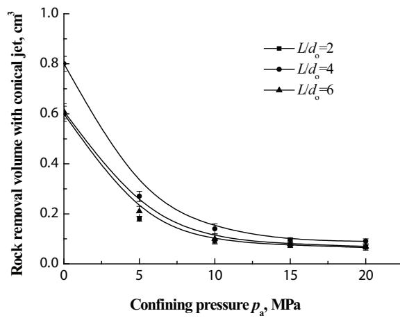
FIG. 6: Rock removal volume by conical nozzle #1 varies with confining pressure.
