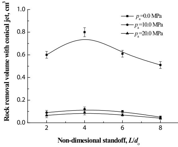
**FIG. 7:** Rock removal volume by conical nozzle #1 at different standoffs.
